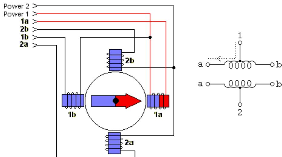
Conceptual Model of Unipolar Stepper Motor
